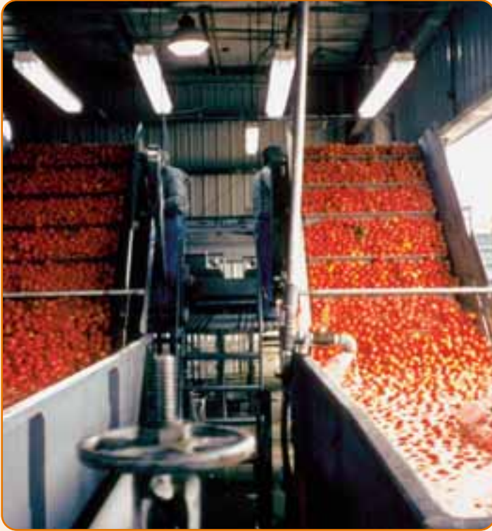
5998 FLUSH GRID BELT FOR FRUIT APPLICATIONS
