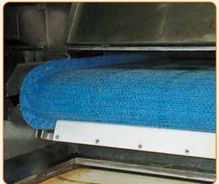
6391 FLUSH GRID BELT FOR BLANCHING APPLICATIONS
