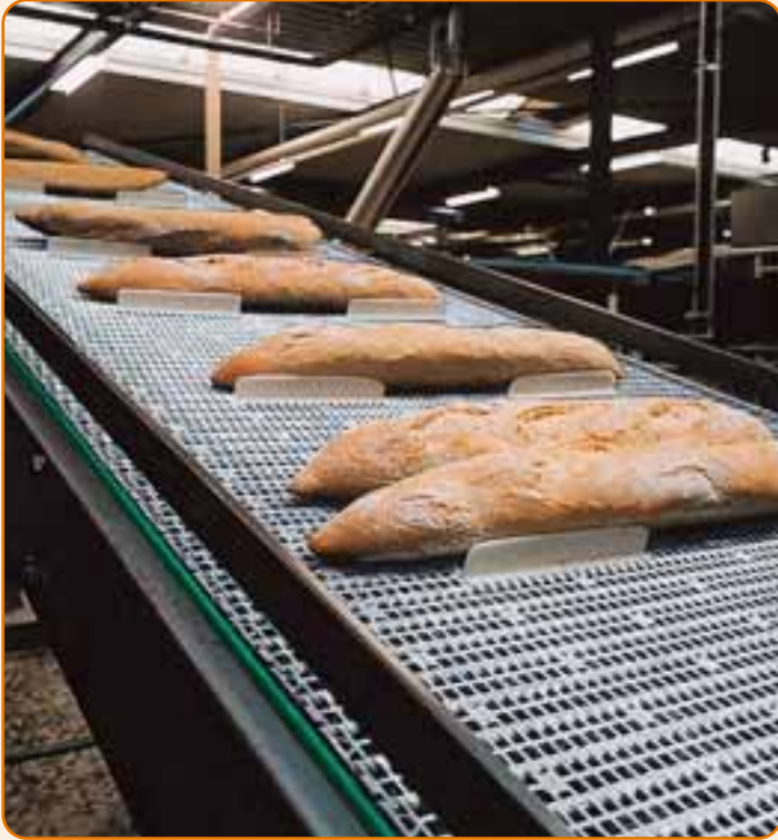
1000 FLUSH GRID BELT FOR BAKERY APPLICATIONS
