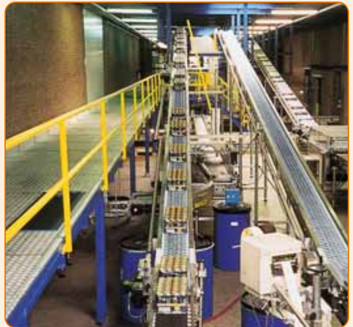
TRAYS WITH CANS SMOOTHLY CONVEYED ON 1000 SUPERGRIP
