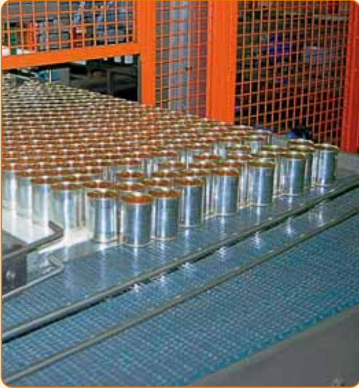
TRANSFER OF CANNED FOOD FROM 1505 FLAT TOP BELT TO 1000 FLUSH GRID BELT
